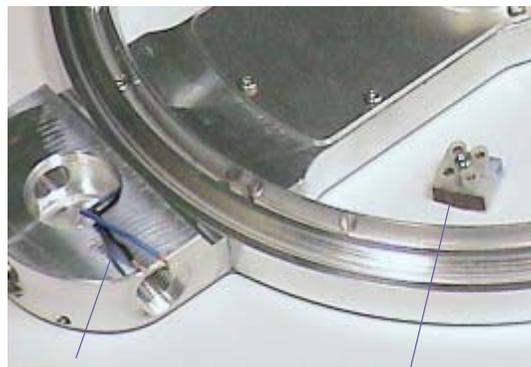
Motor pigtail Terminal block(removed)
